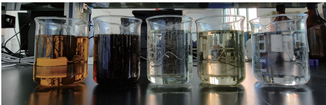
▲ Ultrafiltration & Nanofiltration Salt Separation Photos (Feed, Ultrafiltration Concentrate, Ultrafiltration Permeate, Primary Nanofiltration Concentrate, Secondary Nanofiltration Permeate).
