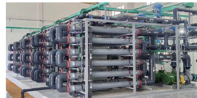
▲ 400 m 3 /h Circulating Water Blowdown Treatment Project for a Photovoltaic Company in Yunnan (Total Water Recovery Rate >90%)
