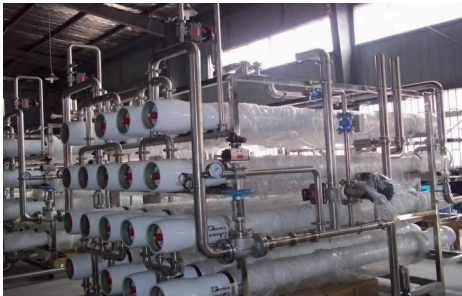
▲ 10 m³/h (20% sugar content) Continuous Purification Filtration Equipment for High Fructose Syrup
