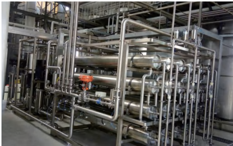
▲ 9 m³/h (25% sugar content) Continuous Purification Filtration Equipment for High Fructose Syrup
